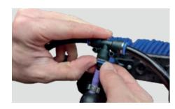
viii. Simply push in the purple button on the brush to release it from the angle adapter at the top of the pole.
