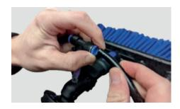
v. You can choose where you want your jets to be, which we place on the edge of the brush which you push your jet nozzles in and you simply twist and lock using the twist mechanism, turning clockwise.
