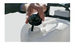
iv. Insert your AHA-H6 telescopic pole hose directly to the water outlet connection. This will give you an extra 15mtr of hose which maybe required in tight areas
