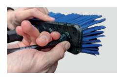
iii. It is important to make sure there is a firm seal around the hose to help protect leakage. To make sure the hose is attached correctly when you push the hose into the tee-piece you should hear a click sound and then push it in a second time to make sure its fully secure. You can check by trying to pull the hose out the tee-piece.
