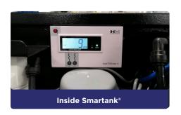
2) The second TDS meter is mounted on the front of the Smartank® cabinet, which monitors the water purity of both DI filters (operator 1/operator 2). If the final water reading is above 5ppm, a replacement DI filter is needed
