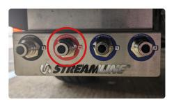
3. Switch the solenoid valve 'on' with the solenoid switch to fill. The controller will monitor the level switch in the water tank and fill the tank by energising the solenoid filling valve. When the water level rises and operates the level switch, the controller will de-energise the solenoid filling valve and stop the filling process automatically
