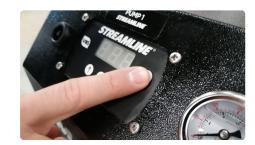
3. You can adjust the water flow rate by increasing/decreasing the flow rate number until a desired flow rate is achieved. The average flow rate is usually set between 40-50 on the Streamline™ controlers (approx. 2.5lpm). The pump MUST run continuously. If the pump is running intermittently whilst water is flowing to the telescopic pole, decrease the speed on the flow controller by pressing the button until the pump runs continuously.
