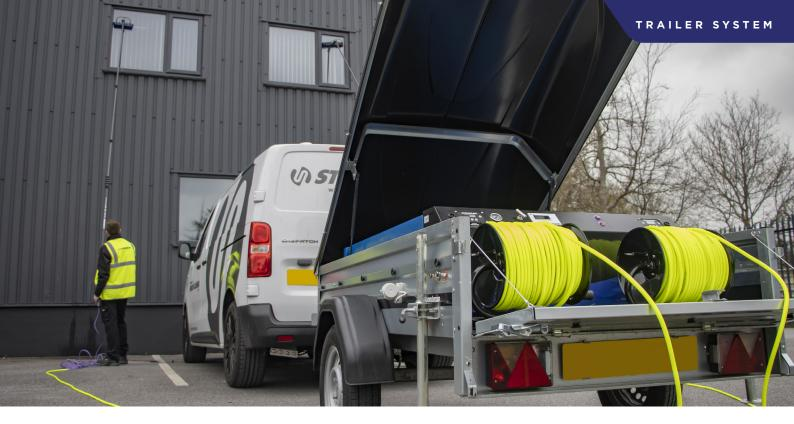
Using the Smartank® flat tank 400Ltr system, the baffled tank ensures the low centre of gravity maximises the stability during transportation. With the equipment cabinet mounted at the front of the tank, at the door opening, operation has never been easier...
