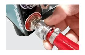
iv. Connect the 2x BLUE hose from the pure water outlet to your waterfed poles (it is possible to add a Streamline® 100mtr hose reel)
