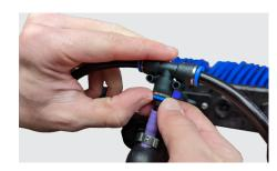
**viii.** Simply push in the purple button on the brush to release it from the angle adapter at the top of the pole.
