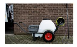
ii. Remove the container lids and riser tube and fill the container with pre-filtered water. If the trolley is fitted with a resin filter fill the container with tap water.
