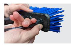
iii. It is important to make sure there is a firm seal around the hose to help protect leakage. To make sure the hose is attached correctly when you push the hose into the tee-piece you should hear a click sound and then push it in a seccond time to make sure its fully secure. You can check by trying to pull the hose out the tee-piece.
