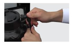
**iii.** Unscrew the filter bracket and remove the DI filter from the trolley.
