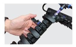
**ii.** Secure the extended section by closing the clamp lever fully. Continue to lengthen the pole by extending each section, one at a time, until the desired height is achieved.
