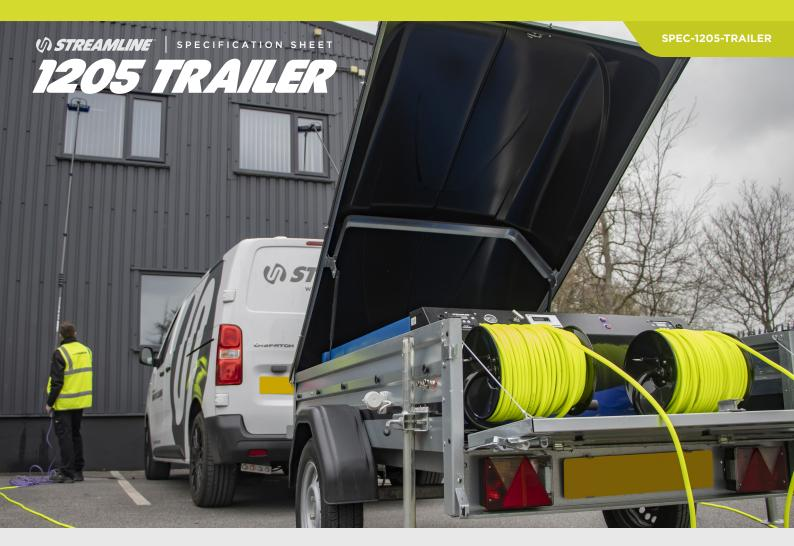
The small compact BrenderUp 1205 trailer system is an excellent trailer system for on-site and on road. With 13" wheels for ease of towing, lockable ABS lid, gas struts, jockey wheel and tailgate as standard, this is a high-quality trailer specification. As the trailer is unbraked, and 750kg gross payload, there is no BE+1 license required in the UK.
